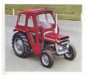
An attractive cab, specially designed by Massey-Ferguson, combines pleasing appearance with great comfort and convenience. The steel-framed fibre-glass construction is draught-free, rain proof and rust proof. The driver has full access to implements and has plenty of room inside. The top and side doors are easily removed in warm weather, while an optional roller blind with inset window provides maximum protection at the rear during the winter months.
