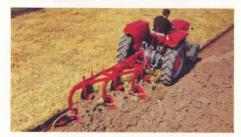
Position Control lowers the links to any desired height. It's invaluable when doing repetition work such as drilling post holes. Set the control lever stop to the desired position and every hole is made to the same depth. Also helpful when hitching heavy implements, or for controlling the working of semi-mounted equipment such as small levelling blades or rotary cutters.
