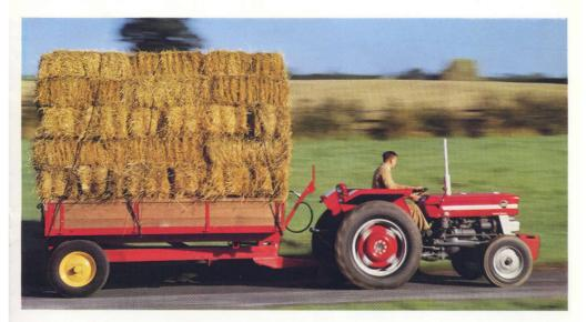
Multi-Power — Massey-Ferguson's exclusive change-on-the-go gear shift — gives twelve forward speeds and four reverse. In Multi-Power High range you get an extra 30% of speed — on the road you can travel at up to 20 m.p.h. Simply select the gear you want, then use Multi-Power to flick from High to Low at the touch of a switch.
