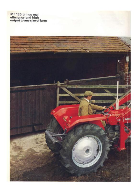
Underneath the compact dimensions and beautiful styling, the famous MF 135 tractor is rugged and powerful. The engine — an economical 45.5 h.p. 3-cylinder diesel — is built by Perkins to MF specifications. It has been proved in hundreds of thousands of tractors all over the world. The MF 135 is built at Coventry — at the world's most
